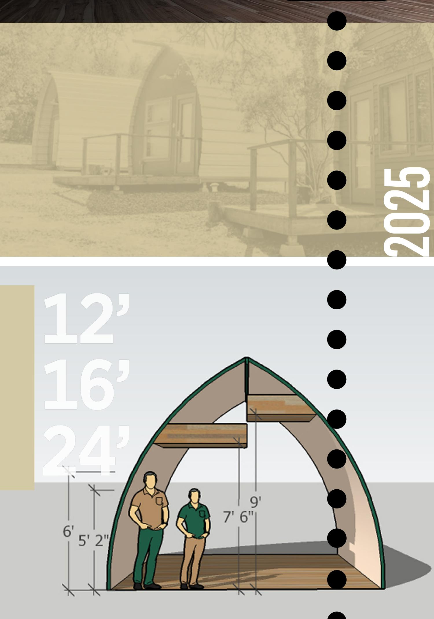
Structural steel "ribs" run every two feet down the length of the cabin making our Arched Cabins even stronger than traditional framed houses. **Preferred lengths for the T12 are** 16', 20' and 24'. Custom lengths available up to 46'
