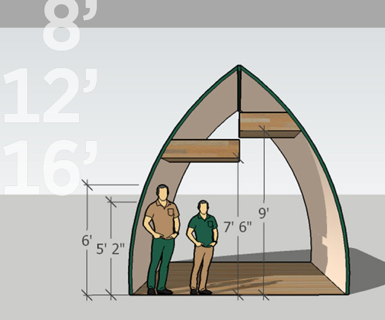
Structural steel "ribs" run every two feet down the length of the cabin making our Arched Cabins even stronger than traditional framed houses. Preferred lengths for the T8 are 8', 12', and 16'. Custom lengths available up to 46'.
